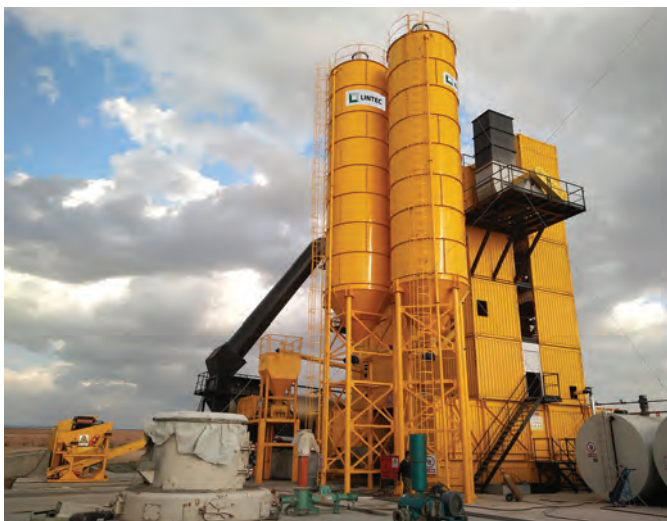
The Lintec CSM series of asphalt plants is built in ISO certified sea containers for economical shipment and fast installation and dismantling.
