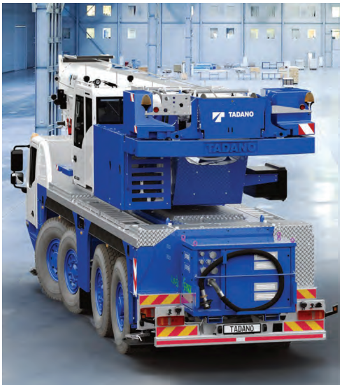
Tadano AC 4.080-1 all-terrain crane equipped with E-Pack.
