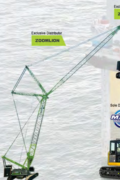
Crawler Crane with luffing jib
