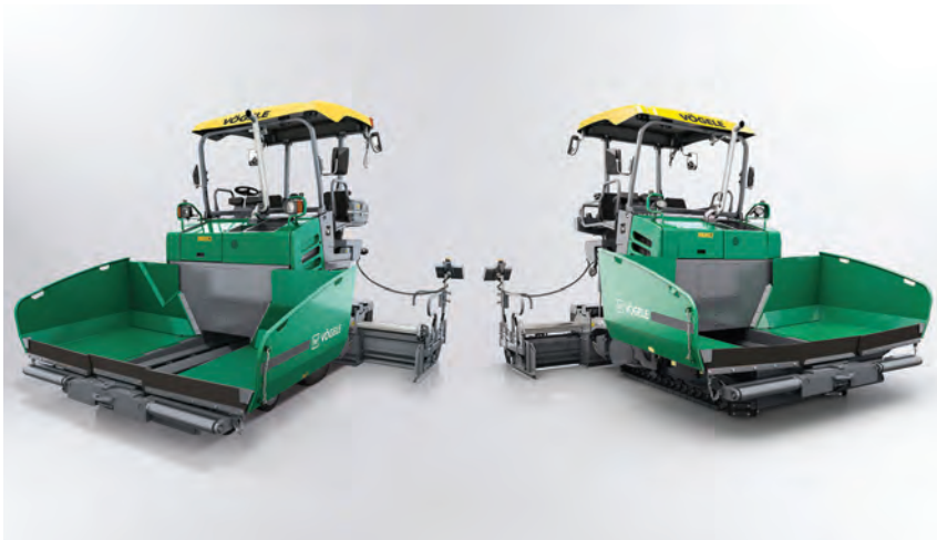
Vögele's new Super 1303 wheeled paver (left) and Super 1300 tracked paver have laydown rates of up to 350 t/hr, and pave widths from 0.75 to 5 m. Featuring a compact design, the machines are ideal for small to medium-sized projects.
