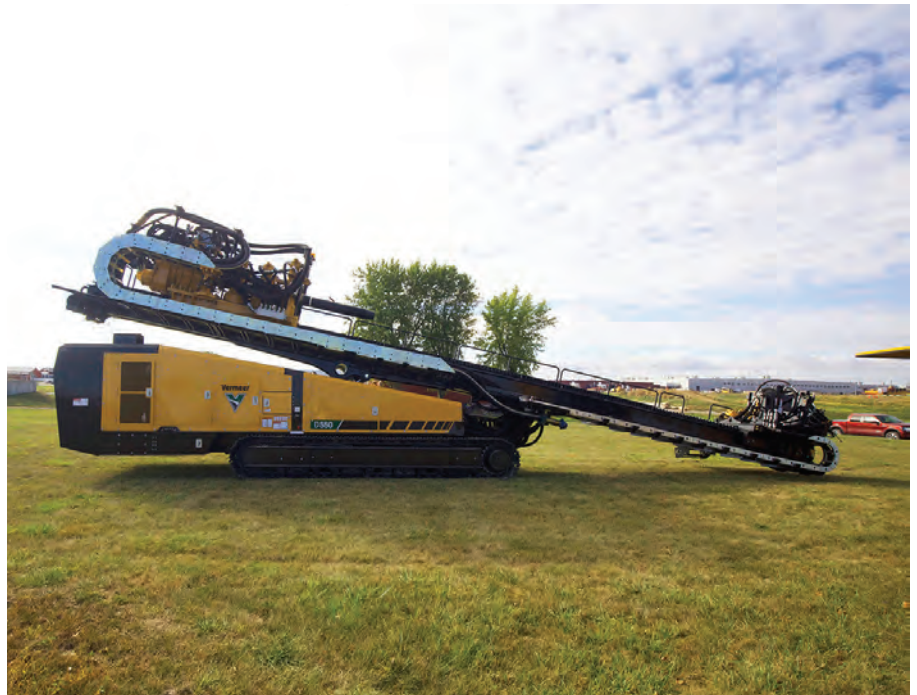
The new Vermeer D550 HDD features 135,581 Nm of torque, advanced telematics, and smart onboard technology and diagnostic information. The machine is suitable for installing large-diameter products, such as oil and gas pipelines, water lines and high-voltage electrical transmission lines at long distances.
