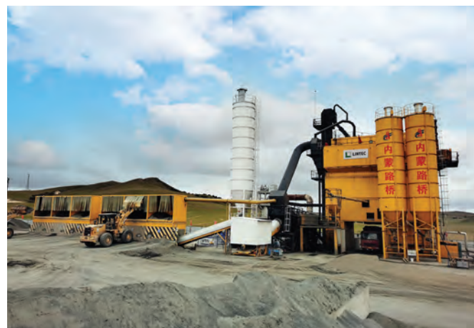
The Lintec CSM4000 asphalt plant was subsequently procured for the construction of the Jingwu Expressway after seeing the success of the CSM5000 plant on the G65 BaoMao Expressway project.
