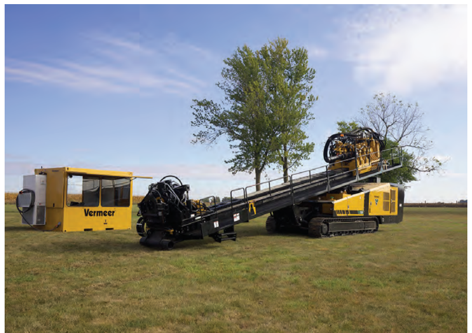
The D550 HDD also features many mechanical enhancements, including a full travel vise, engineered hydraulic transmission and quiet engine. The full travel vise can be positioned up and down the rack as needed for making/breaking tooling and optimising efficiency during casing installation.
