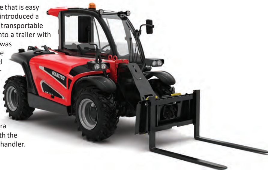
ABOVE AND LEFT: The compact machine features a width of just 1.49 m and a height of 1.92 m.
